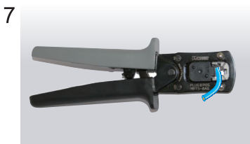
7 Using special crimping tool MPT5-8AS (PANDUIT CORP.), crimp the modular plug. Finally, check the plug visually.
